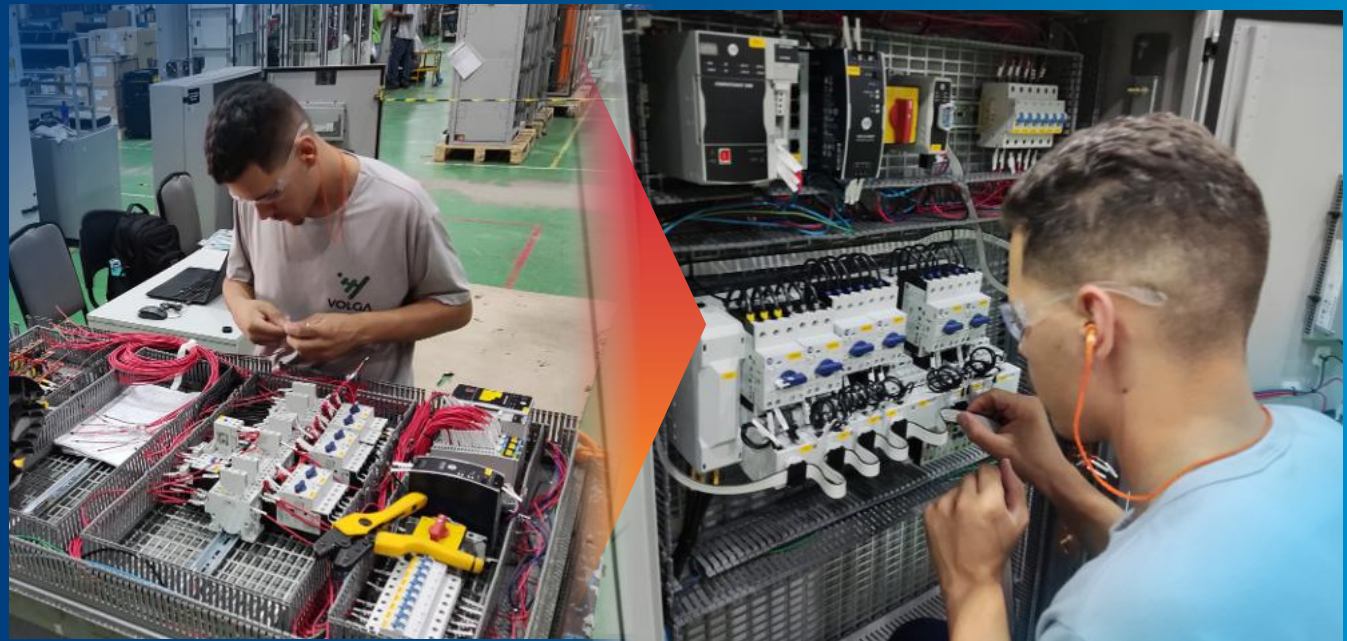
Traditional hardwired panel Over 20 hours to wire
